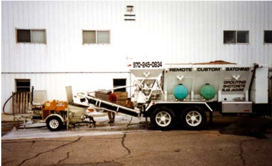
On site batching of zero slump grout using a high-pressure pump equipment.
